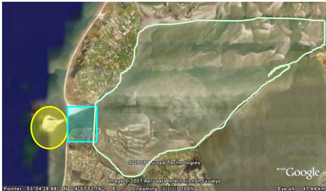
Figure 2-1: Different components of Marsdiep Tidal inlet system in Dutch Wadden Sea: Ebb-tidal Delta (Yellow), Tidal inlet (Blue), Tidal Basin (Green)
