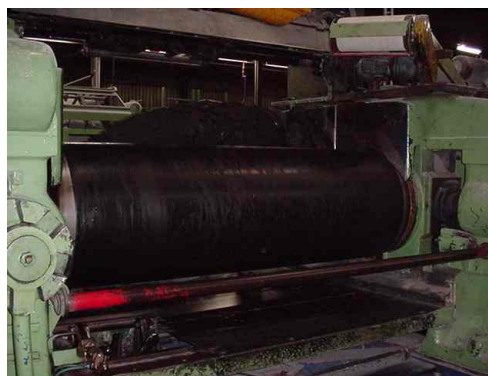
Fig 12.2 RubbERMENGSSEL in mengmolen
