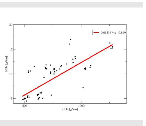
Figure 4: the relation between  $NO_x$  and  $CO_2$  for all the city measurements. The slope indicates a relation of about 13 g  $NO_x$  per kg  $CO_2$ Originally the relation between  $NO_x$  and  $CO_2$  was estimated at 8.5-9.0g  $NO_x$  per kg  $CO_2$ .
