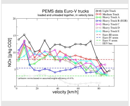
Figure 2: Results of the PEMS measurements on EURO V trucks.
