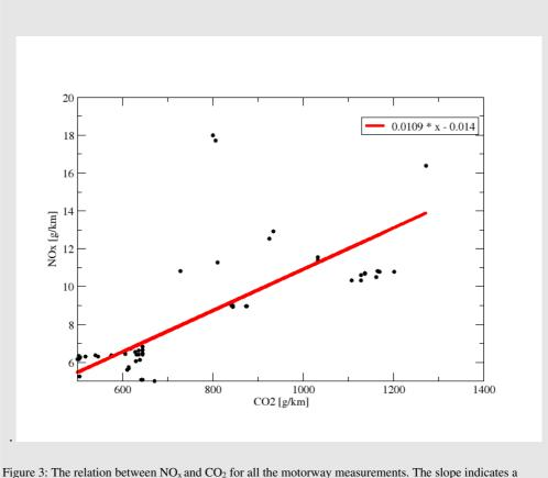
Figure 3: The relation between NO<sub>x</sub> and CO<sub>2</sub> for all the motorway measurements. The slope indicates a relation of about 11 g NO<sub>x</sub> per kg CO<sub>2</sub>. Originally the relation between NO<sub>x</sub> and CO<sub>2</sub> was estimated at 8.5-9.0 g NO<sub>x</sub> per kg CO<sub>2</sub>.
