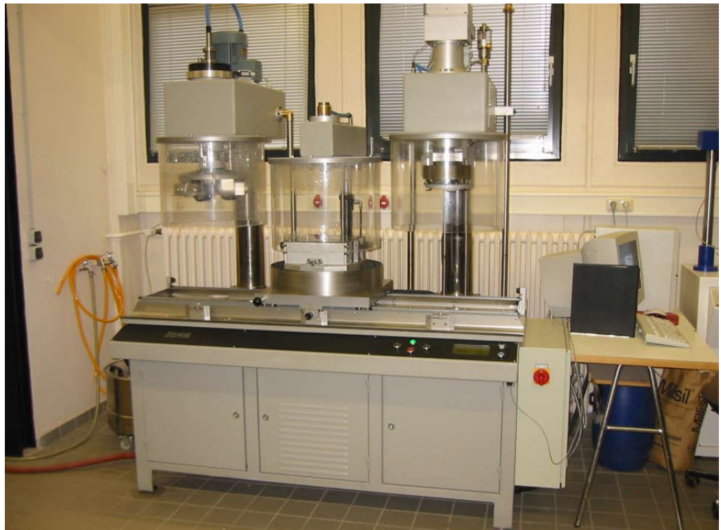
Figure 1: Set-up for Wehner/Schulze test
