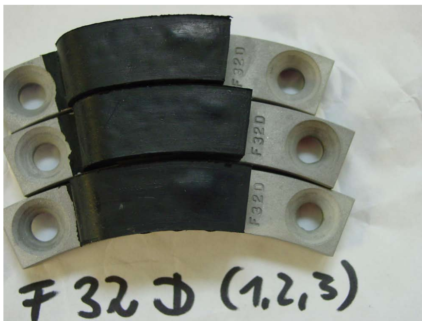
Figure 3: Blisters on the test rubbers
