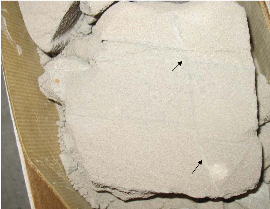
Figure 2-15 Anhydrite-healed small-scale faults in core 11 of BGM1.
