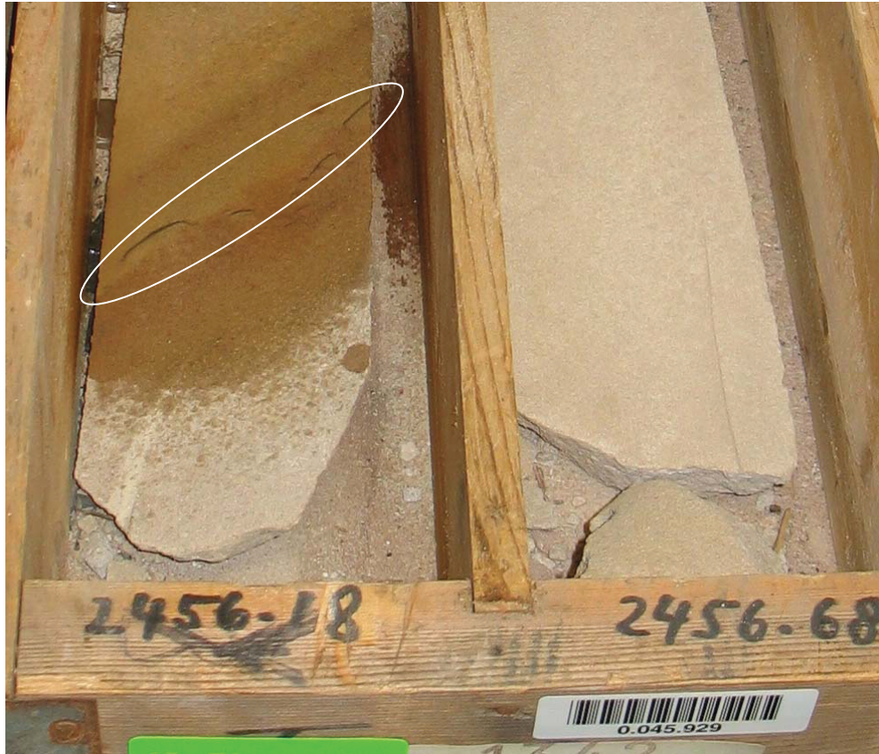
Figure 2-9 Mud flakes suggest fluvial influence in the upper part of the GRT3 cores.
