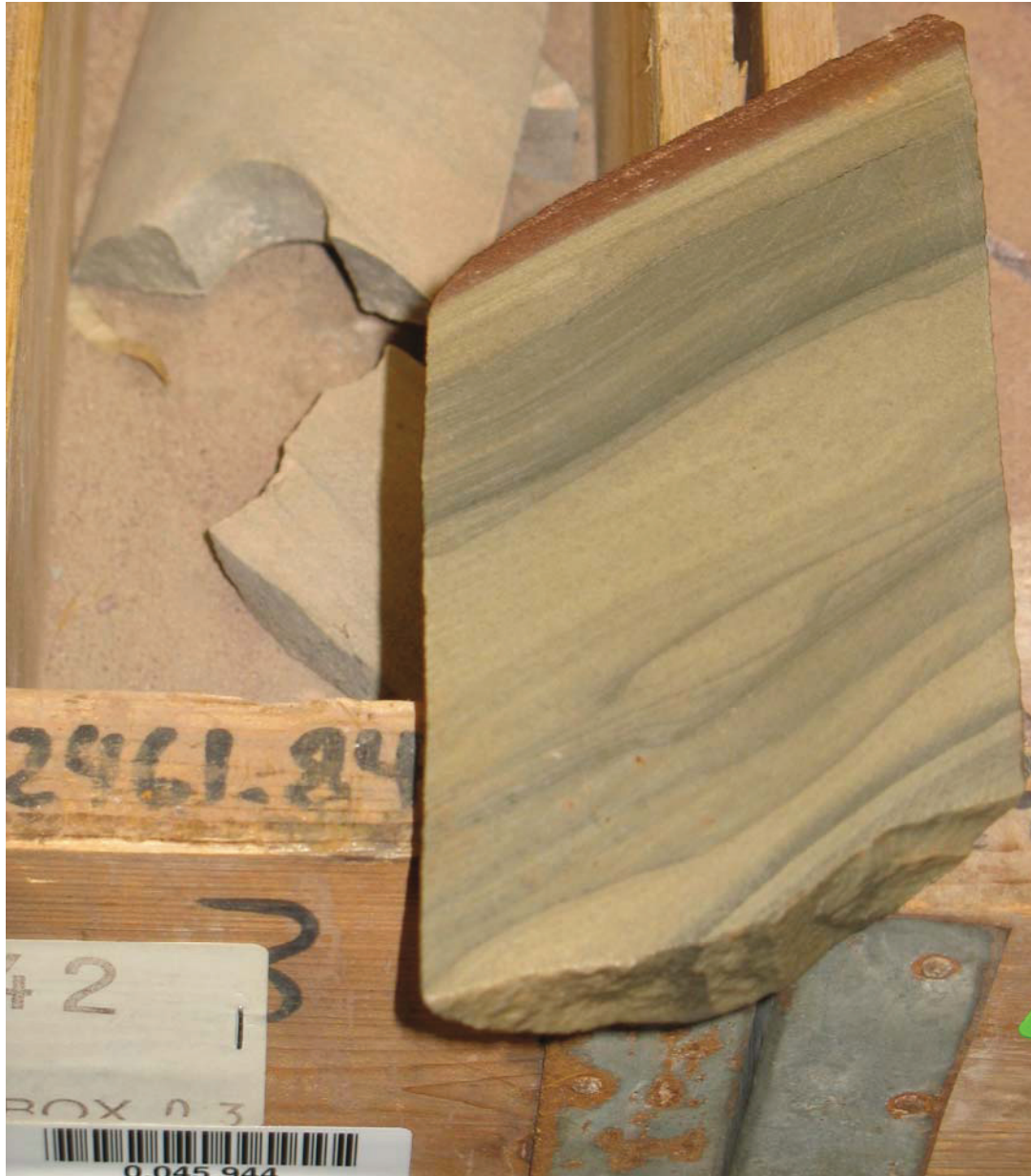
Figure 2-8 Fluvial water ripples in GRT3. The core sample is from 2462m MD, the overall thickness of this fluvial interval is about 15cm.
