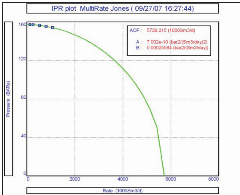
Figure 3-1 IPR plot BGM-1 using isochronal test results of 1979.
