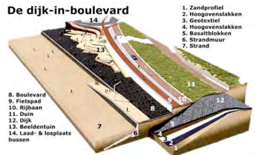
Figuur 6: De Dijk-in-boulevard in Scheveningen
