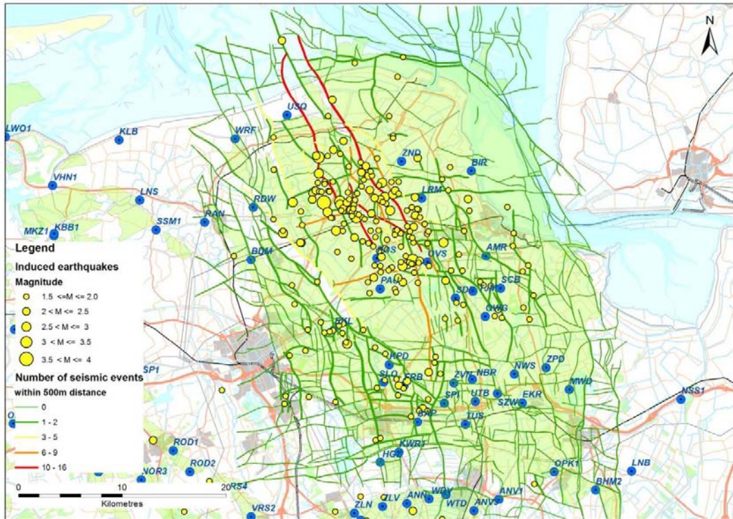
Figure 9.6 Groningen fault map with epicenters of recorded seismic events > 1.5 . Color of faults indicates the number of events within 500 m distance from each fault. A selection of wells drilled in the area is indicated by the blue dots. Faults shown are at Top_Rotliegend level
