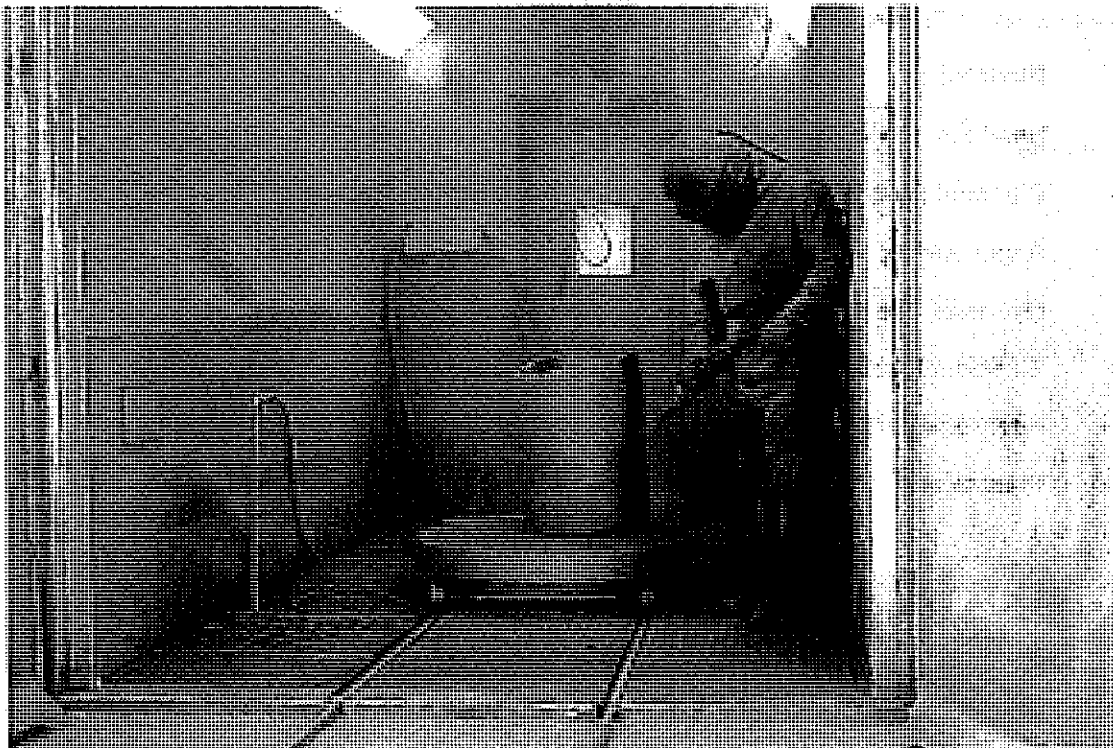
Figure 7-2: Dry blasting decontamination (Picture by courtesy of EWN)
