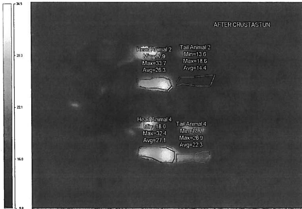
Figure 4. Thermal images of a second group of four langoustines after being killed using the Crustastun machine. In this case there was some change in the temperature of at least two of the tails. Values refer to the outlined areas.
