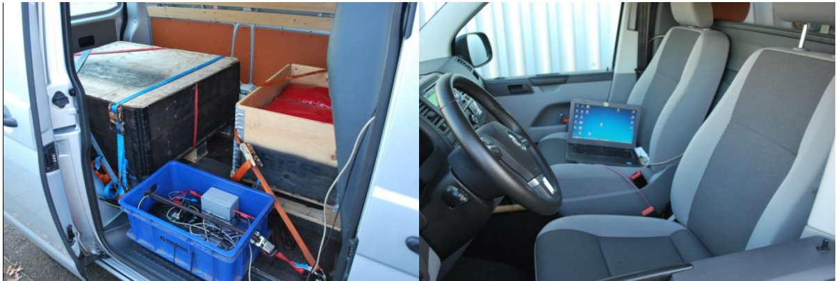
Figure 9: Left: Load packages (black box) and data logger of the SEMS (blue cradle) used in on-road testing of a light commercial vehicle. Right: The laptop used to monitor and control the SEMS equipment.
