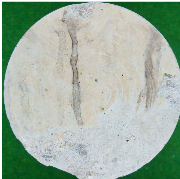
Figure 9: Photo of the surface of core M66-K9. The surface is plane and smooth. Part of the surface has broken off, which probably happened when taking out the core.
