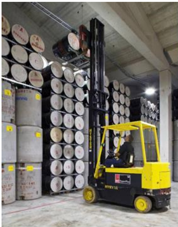
Figure A.2 The storage of low- and intermediate-level waste in the LOG
