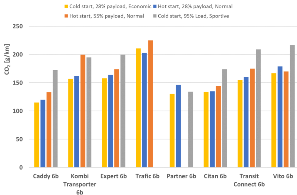
Figure 3-61: CO 2 emissions of RDE trips with different payloads and driving styles of 8 vehicles
