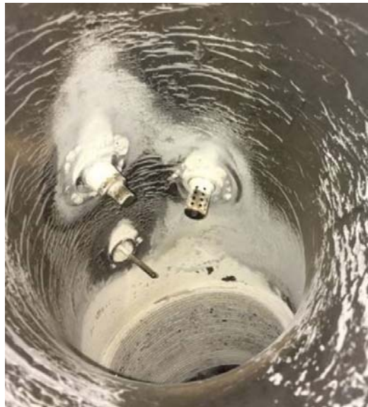
Figure 4: White deposit was observed in the tail-pipe of vehicle DA173.
