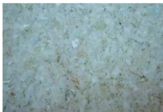
2 nd pass natural HDPE from S+S trial (96% purity)
