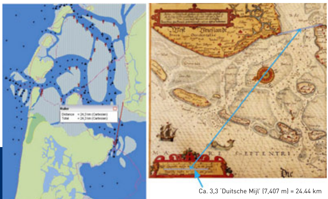
FIGURE 3: Check of reference distances on the map in modern projection (left) and on the original map (right).
