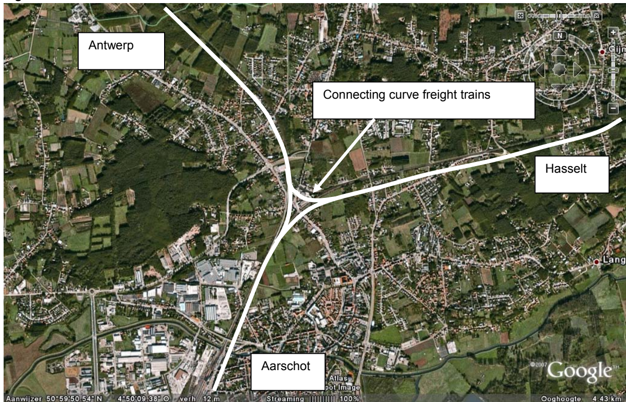
Figure 35: Aerial view of the situation of the Aarschot bottleneck
