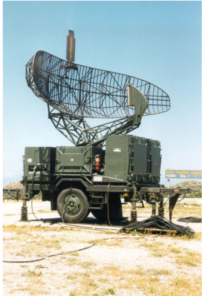
FIGURE 1 – Example of HAWK radar: the PAR (Pulse Acquisition Radar). [Color figure can be viewed in the online issue, which is available at www.interscience.wiley.com .]
