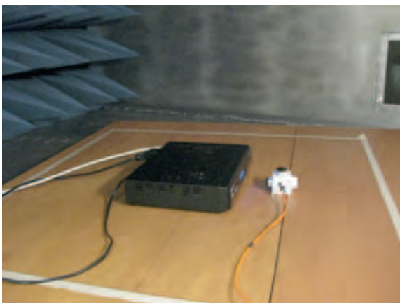
Figure 4 and 5. Sensor near set-top box and television set in GTEM
