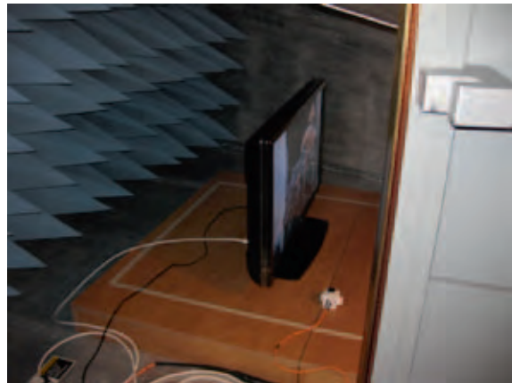
Figure 4 and 5. Sensor near set-top box and television set in GTEM
