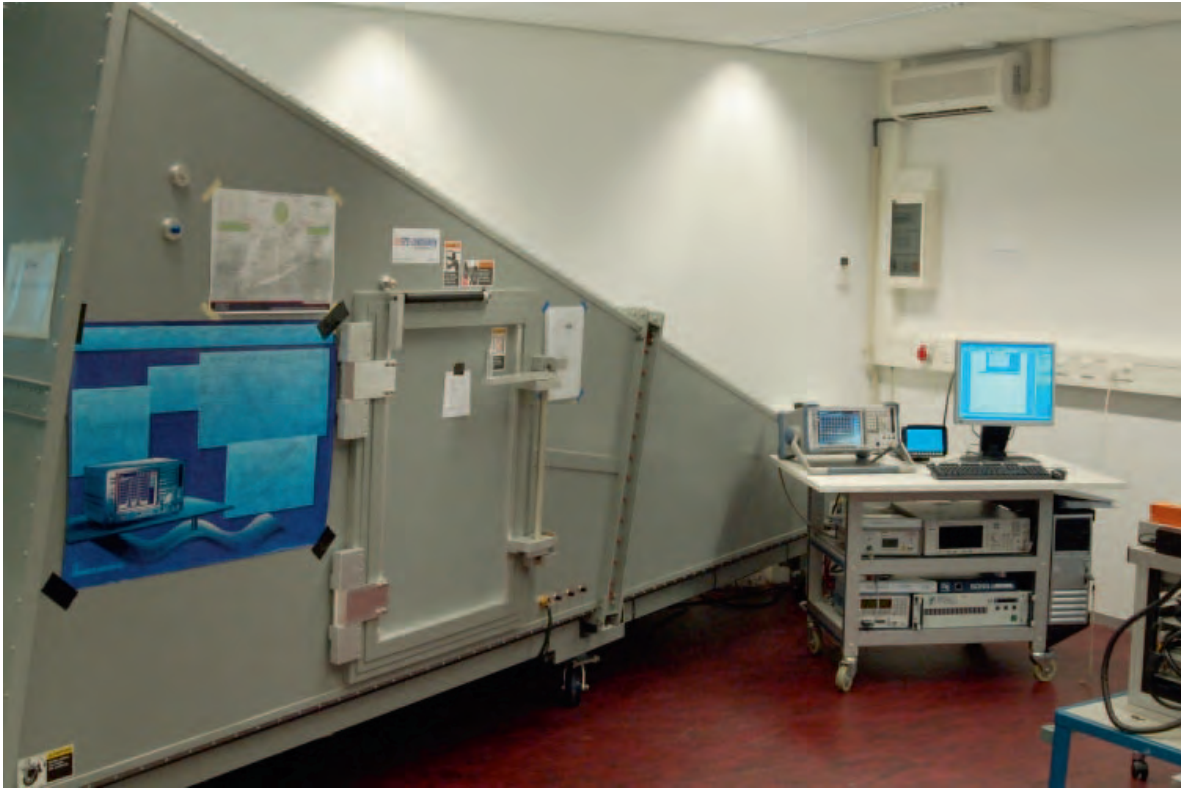
Figure 3. Setup for testing immunity; GTEM (Gigahertz Transverse Electromagnetic Cell)
