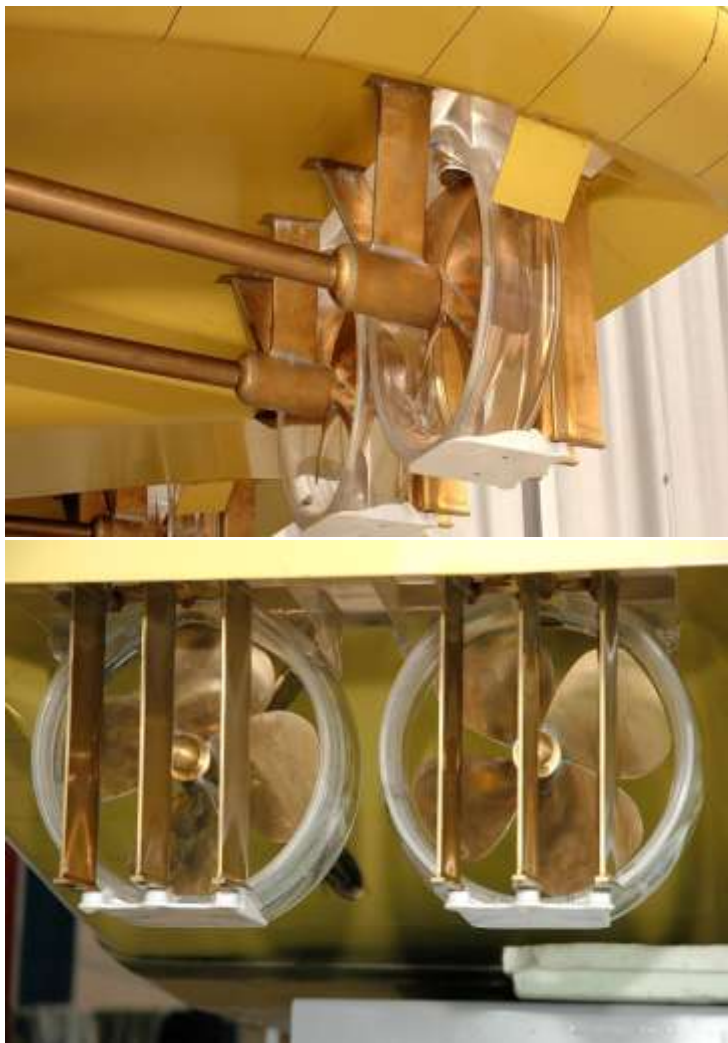
Figure 15: Propeller in nozzle with fixed shafts and rudders
