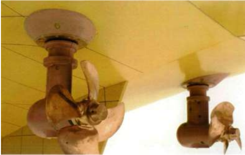
Figure 17: Azimuthing thrusters with open pushing propellers
