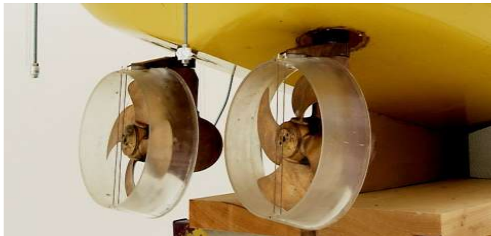
Figure 16: Azimuthing propellers with propellers in nozzles
