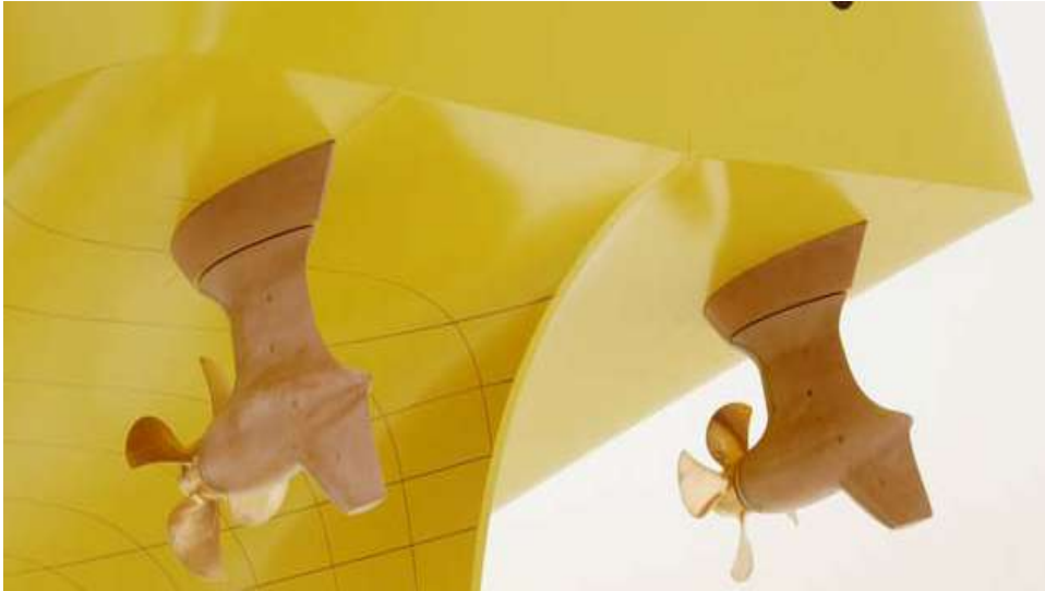
Figure 21: Azimuthing thrusters with open pulling propeller
