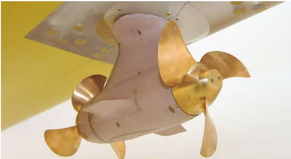
Figure 22: Azimuthing thrusters with tandem propellers (rotating in the same direction)
