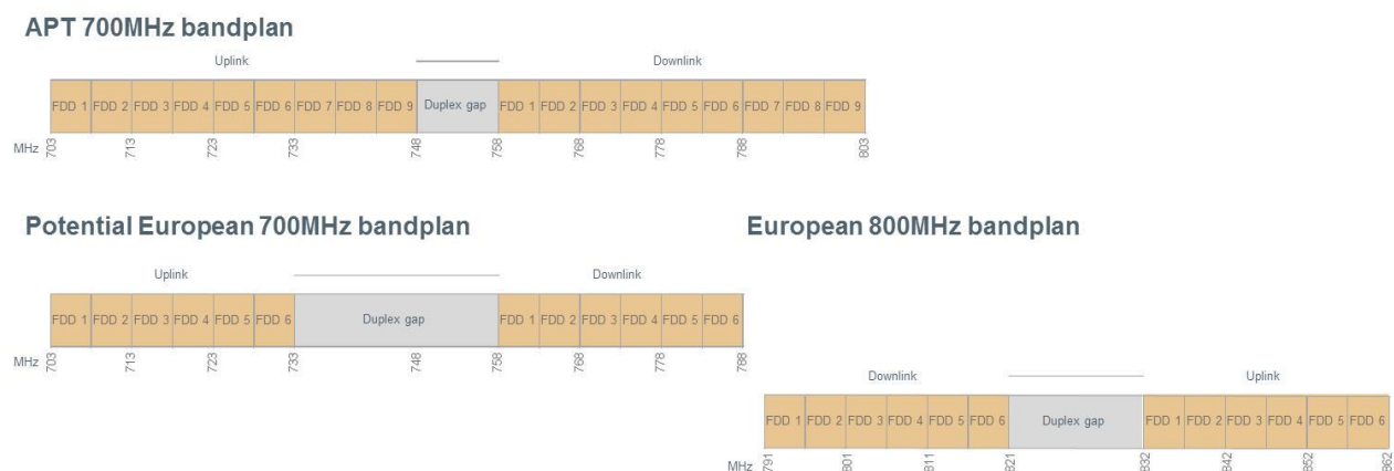
Figure 5-3: Potential alignment of European 700MHz bandplan with APT 700MHz bandplan and European 800MHz bandplan
