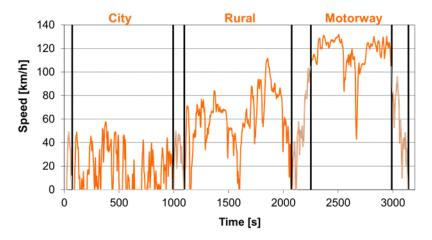
Figure 2-2: Common Artemis Driving Cycle (CADC).
