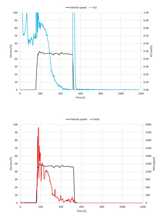
Figure 10-18: PTI chassis dynamometer O<sub>2</sub> and NOx emission test at low idle speed, 50 km/h and low idle speed of the Volkswagen Golf.
