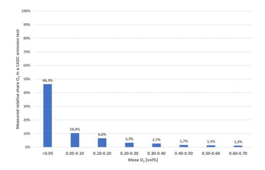
Figure 10-3: Measured relative shares of the  $O_2$  concentration in exhaust gas of a CADC test of the Ford Focus.
