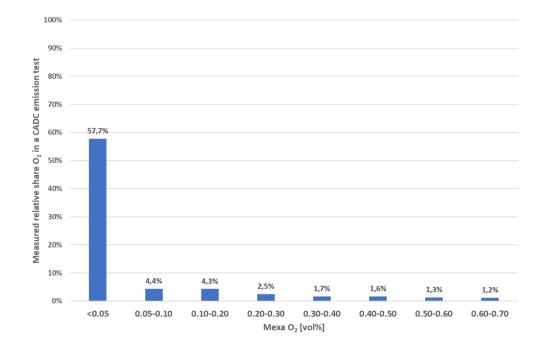
Figure 10-2: Measured relative shares of the  $O_2$  concentration in exhaust gas of a CADC test of the Toyota Aygo.
