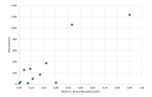
Figure 4-5: Relationship of measured volumetric O<sub>2</sub> concentration at low idle speed and the CADC NO<sub>x</sub> emission in mg/km of the twelve tested vehicles.
