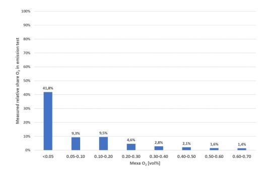
Figure 10-15: Measured relative shares of the  $O_2$  concentration in exhaust gas of a CADC test of the Kia Picanto
