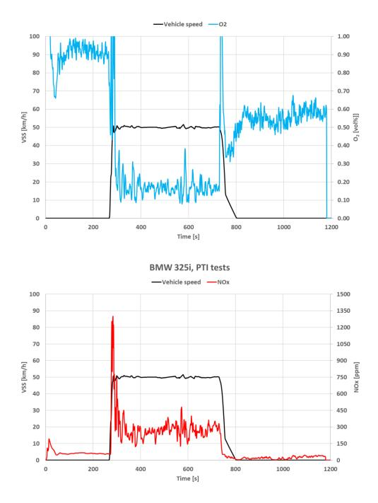
Figure 10-14: PTI chassis dynamometer O<sub>2</sub> and NOx emission test at low idle speed, 50 km/h and low idle speed of the BMW 325i.
