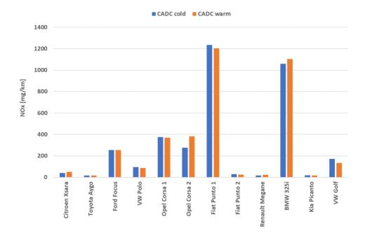
Figure 3-9:  $NO_x$  emission of twelve gasoline vehicles with high mileages in CADC tests with cold and warm start
