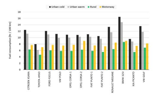
Figure 3-2: Fuel consumption of twelve gasoline vehicles with high mileages in urban conditions with cold and warm start, rural and motorway conditions of a CADC emission test.
