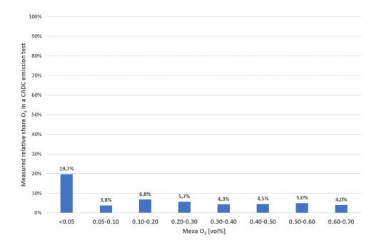
Figure 10-6: Measured relative shares of the  $O_2$  concentration in exhaust gas of a CADC test of the Fiat Punto 1.
