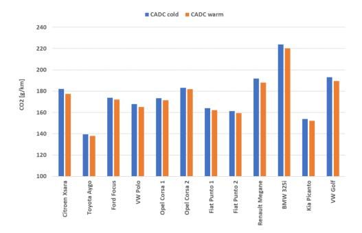
Figure 3-3:  $CO_2$  emission of twelve gasoline vehicles with high mileages in CADC tests with cold and warm start
