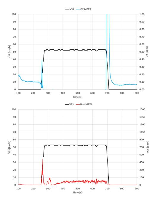
Figure 10-10:  $O_2$  and NOx emissions in a simple emission test at low idle speed, 50 km/h and low idle speed of the Opel Corsa 2
