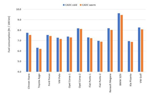
Figure 3-1: Fuel consumption of twelve gasoline vehicles with high mileages in CADC tests with cold and warm start
