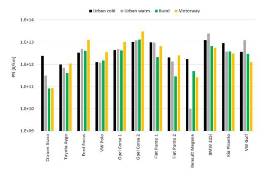
Figure 3-12: Particulate Number (PN) emission of twelve gasoline vehicles with high mileages in urban conditions with cold and warm start, rural and motorway conditions of a CADC emission test.
