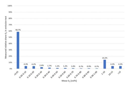
Figure 4-3: Distribution of measured oxygen concentrations in exhaust gas of a CADC test of a stoichiometric gasoline vehicle.
