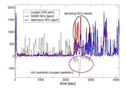
Figure 5-1 The SEMS  $NO_x$  signal should be slightly higher because there is less dispersion of the exhaust gas closer to the engine with the dynamic flow. But between 2200 and 3000 seconds in the test, the oxygen is negative, signalling a rich engine operation, with large deviation of the SEMS  $NO_x$  signal as a result.
