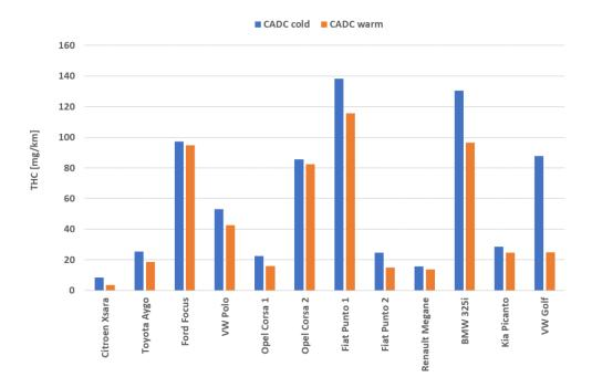
Figure 3-7: THC emission of twelve gasoline vehicles with high mileages in CADC tests with cold and warm start
