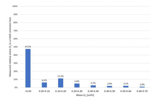
Figure 10-4: Measured relative shares of the  $O_2$  concentration in exhaust gas of a CADC test of the Volkswagen Polo.
