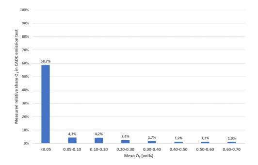
Figure 10-1: Measured relative shares of the  $O_2$  concentration in exhaust gas of a CADC test of the Citroen Xsara.
