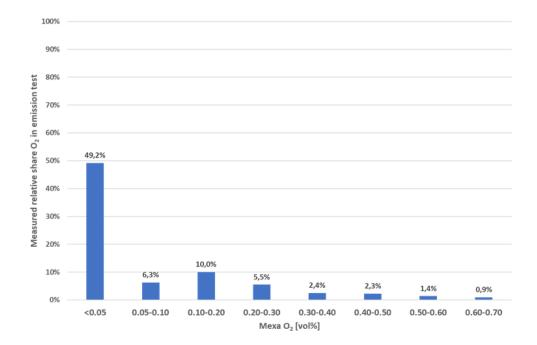
Figure 10-5: Measured relative shares of the  $O_2$  concentration in exhaust gas of a CADC test of the Opel Corsa 1.
