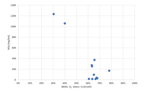
Figure 4-4: Relationship of the measured volumetric CADC O<sub>2</sub> share (< 0.20 vol%) and NOx mass emissions in mg/km of the twelve tested vehicles.
