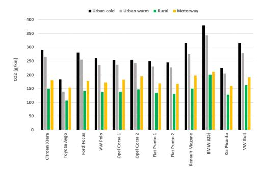
Figure 3-4: CO<sub>2</sub> emission of twelve gasoline vehicles with high mileages in urban conditions with cold and warm start, rural and motorway conditions of a CADC emission test.
