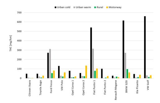
Figure 3-8: THC emission of twelve gasoline vehicles with high mileages in urban conditions with cold and warm start, rural and motorway conditions of a CADC emission test.
