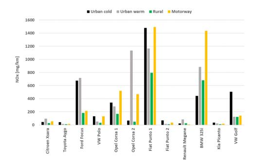
Figure 3-10: NO<sub>x</sub> emission of twelve gasoline vehicles with high mileages in urban conditions with cold and warm start, rural and motorway conditions of a CADC emission test.
