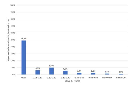
Figure 10-9: Measured relative shares of the  $O_2$  concentration in exhaust gas of a CADC test of the Opel Corsa 2.
