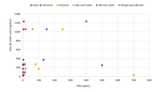
Figure 4-2: Relationship of different NO<sub>x</sub> concentrations of simple emission tests and CADC NO<sub>x</sub> mass emission of the twelve tested vehicles.
