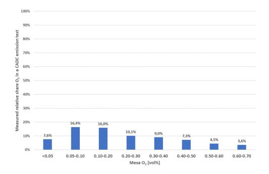
Figure 10-13: Measured relative shares of the  $O_2$  concentration in exhaust gas of a CADC test of the BMW 325i.
