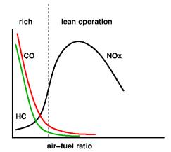
Figure 4-1: The typical emissions of a petrol engine. In lean operation, on the right, NO<sub>x</sub> emissions are high. In rich operation on the left hydrocarbon and CO emissions are high. In between, at the dashed line, HC, CO, and NO<sub>x</sub> are produced in the right balance to be converted in a three-way catalyst into harmless products.
