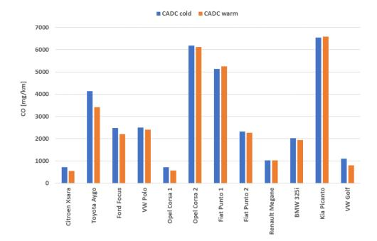
Figure 3-5: CO emission of twelve gasoline vehicles with high mileages in CADC tests with cold and warm start
