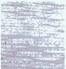
No external materials are added for the welding process. Micrograph shows actual weld line: it appears to be a single consolidated laminate, while it is an induction weld of two parts!
