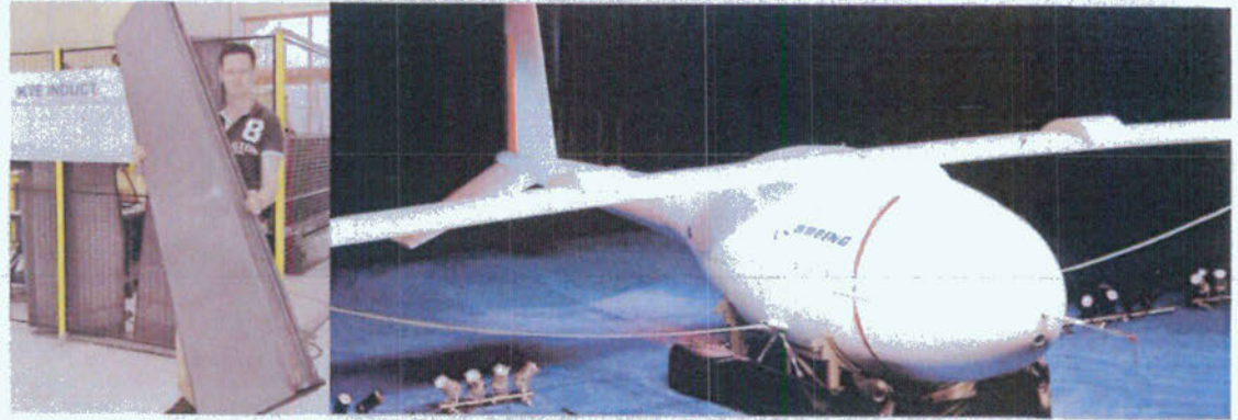
Thermoplastic welded component for Boeing Phantom Eye UAV. Design and build bij KVE Composites
