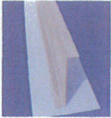
Picture showing a rib which is induction welded to a skin. Both parts in carbon fiber PPS laminates
