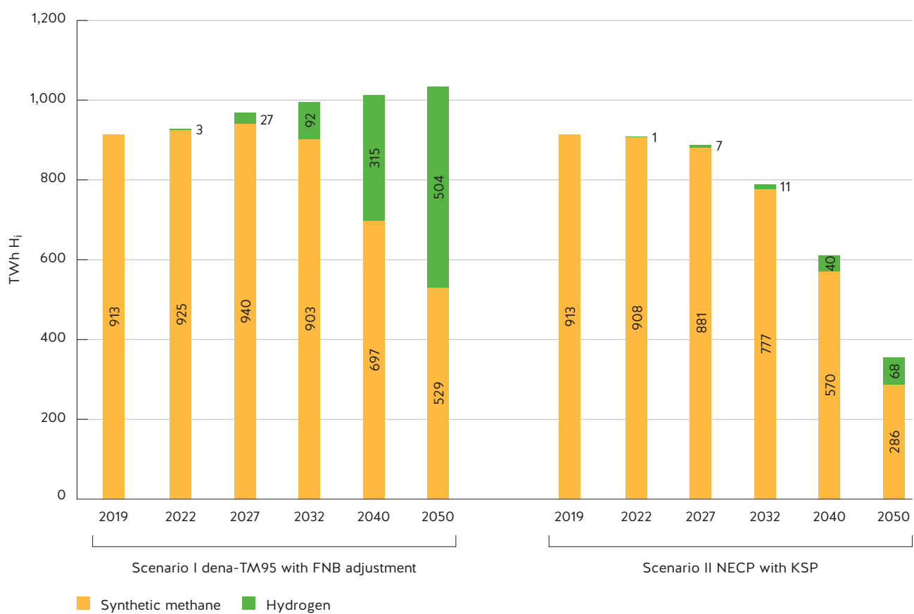
Figure 5: Graphic presentation of the trends in gas demand (methane, hydrogen) in the scenarios considered in more detail up to 2050 in TWh (H i , calorific value)
